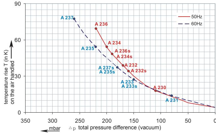
The performance curves are based on air at a temperature of 15 °C and an atmospheric pressure of 1013 mbar with a tolerance of +/- 10 %.
