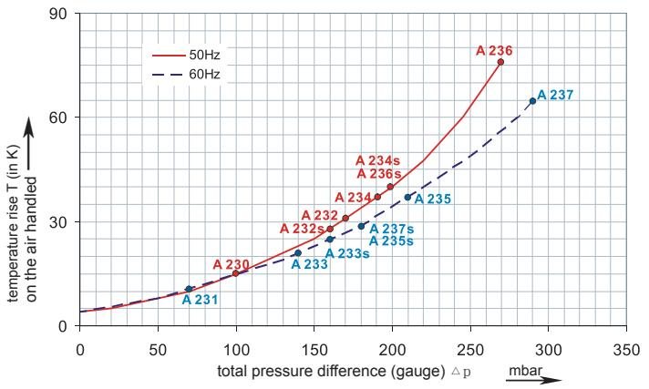
Each G-2RB type can be applied both as vacuum pump and compressor in continuous operation over the total stated performance curve range. The motors are available as standard for the input voltage range of 50 and 60 Hz and for protection category IP 55 as well as approved for UL and CSA.
