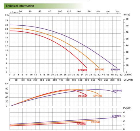
Remarks: Flow curve information based on 220V/50Hz motor.
