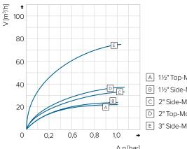
A 11/2" Top-Mount TM 12-ND B 11/2" Side-Mount SM 10-ND C 2" Side-Mount SM 20 D 2" Top-Mount TM 22 E 3" Side-Mount SM 30-ND
