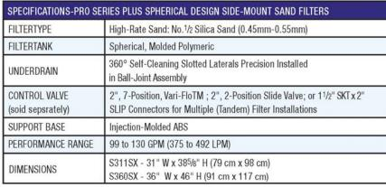
Above dimensions are for filter only. Add 14" (36 cm) for multi-port valve, add 7" (8 cm) for slide valve.
