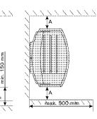
Vega Combi: width 450 mm, depth 385 mm and height 560 mm.
