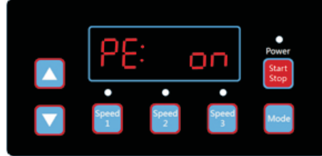
(Diagram 6.23, Self Priming Enable/Disable, default On)
