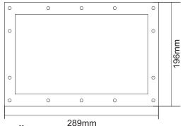
Use the doubled side tape to fix the gasket to the pool wall.
